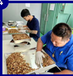
Analysis – Moisture content, Size distribution, Bark and Rotten
